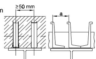
**Connector Positioning (ribs parallel to beam and solid slabs)**
