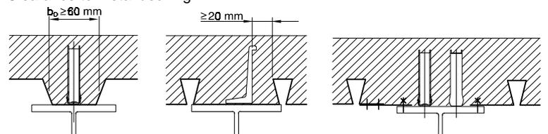
Split decking if necessary for spacing / clearance.
