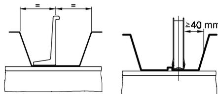
If centering / 40 mm clearance not possible, use minimum of 2 HVB's per rib
