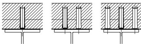
2a. Position in the rib: 1 HVB per rib – leg centered in the rib or 40 mm clearance
