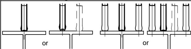
Position the HVB's so that the shear force is transferred symmetrically to the beam.
